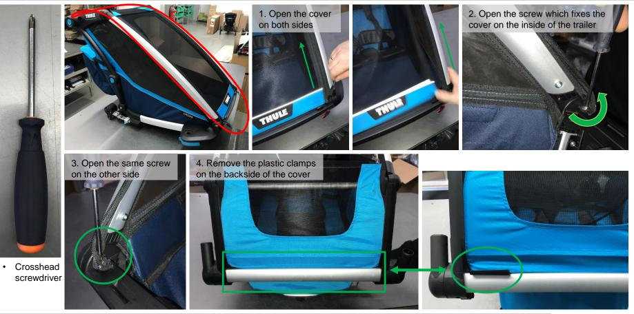
5. Remove the plastic clamps on the backside of the cover and pull out the cover from it's guiding profile
